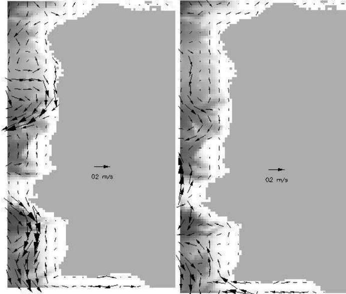
**Figure 5.** Horizontal residual velocity from the PCOMS model at 150 m deep: May-June period (left) and November-December period (right). Note that vectors are represented each four model cells to allow a clearer visualisation.
