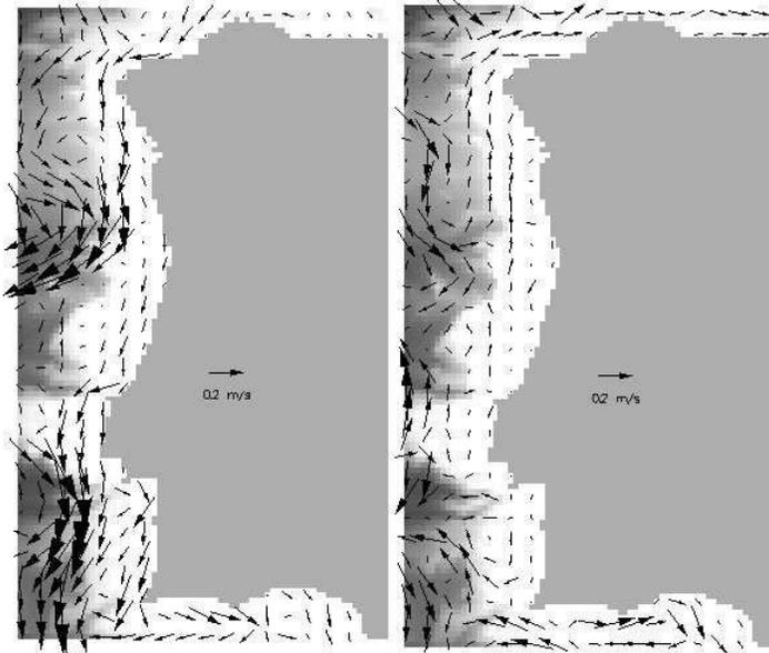
**Figure 3.** Horizontal residual velocity from the PCOMS model at the surface: May-June period (left) and November-December period (right). Note that vectors are represented each four model cells to allow a clearer visualisation.
