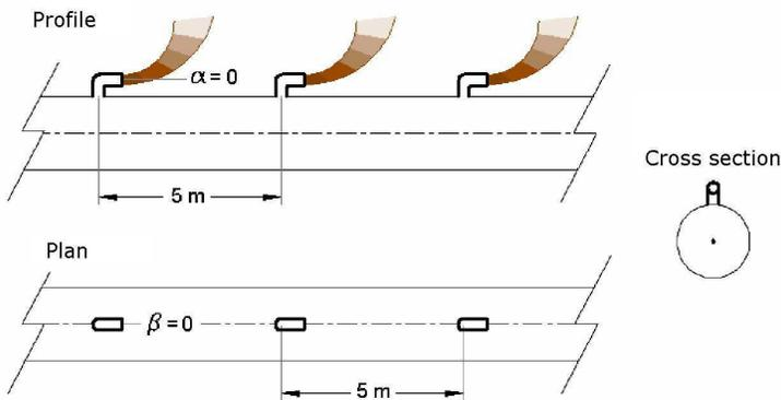
**Figure 7.** Plan view, profile and cross section of the preliminary diffuser design.
