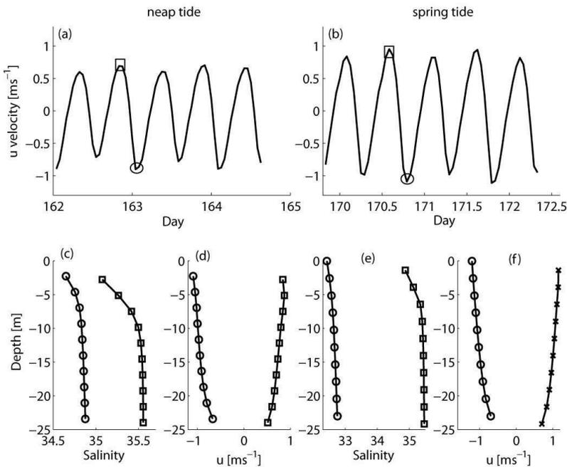
**Figure 2.** Time series of along-channel depth-averaged velocity ( $u$  component) at station A at neap and spring tide for June 2004; (c, d). Vertical profiles of salinity and current velocity at the peak flood (squares) and peak ebb (circles) at neap tide and (e, f) spring tide. (From [22])
