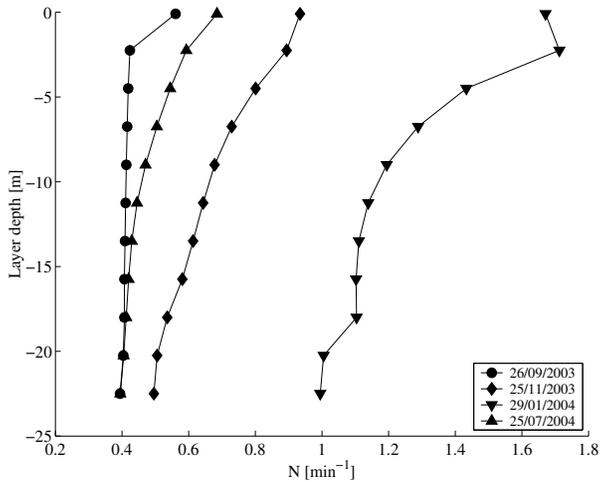
**Figure 5.** Buoyancy frequency,  $N$  ( $\text{min}^{-1}$ ), as a function of layer depth (m). (From [6])
