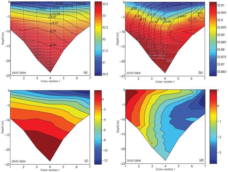
**Figure 4.** (a, b) Cross-sections of tidally averaged salinity (shading) and longitudinal velocity component (contour,  $\text{cm s}^{-1}$ ); (c, d) predicted tidally averaged salt transport ( $\text{cm s}^{-1}$ ) for cross-section 1, near the mouth of the lagoon. (a, c) are for neap tide and river flow of  $143 \text{ m}^3 \text{ s}^{-1}$  and (b, d) are for a neap tide and river flow of  $2 \text{ m}^3 \text{ s}^{-1}$ . (From [6])
