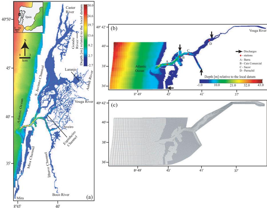
**Figure 1.** (a) Bathymetry of the Ria de Aveiro lagoon and adjacent coastal area. Major tributaries are marked; (b) Bathymetry of the Espinheiro Channel with the discharge points (marked with arrows) and its major freshwater tributary. The location of the stations used in the hydrodynamic calibration procedure is marked. Depths are in meters (over the local datum); (c) Horizontal curvilinear coordinate system [6].
