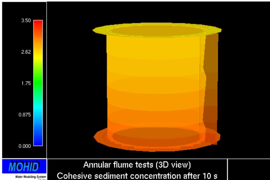
Figure 11 – Cohesive sediment concentration (mg/l) after 10 seconds of simulation with surface stress forcing
