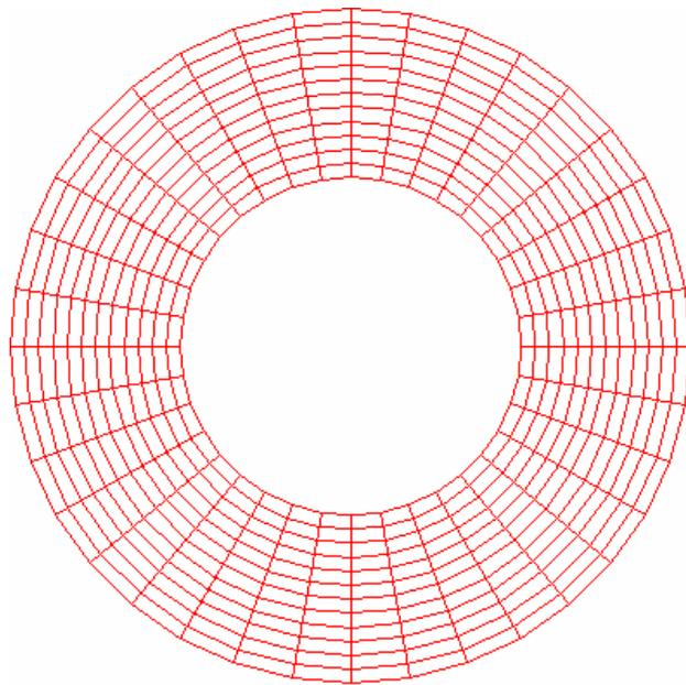
**Figure 2- Horizontal grid discretization**
