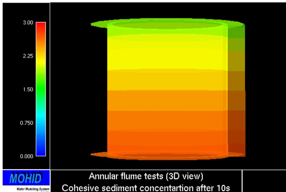
Figure 12 – Cohesive sediment concentration (mg/l) after 10s of simulation with no surface stress forcing
